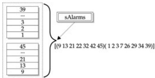
Figure 12–10: The array after it has been partitioned
