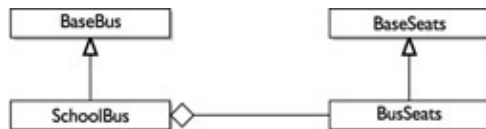
Figure 9–11: The difference between inheritance and aggregation/composition
